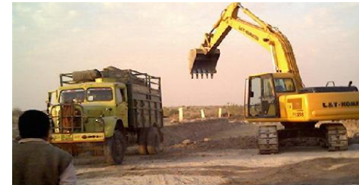
DIRECT EXCAVATION OF GYPSUM AND LOADING INTO TRUCKS DEPLOYED BY THE CONSUMER
